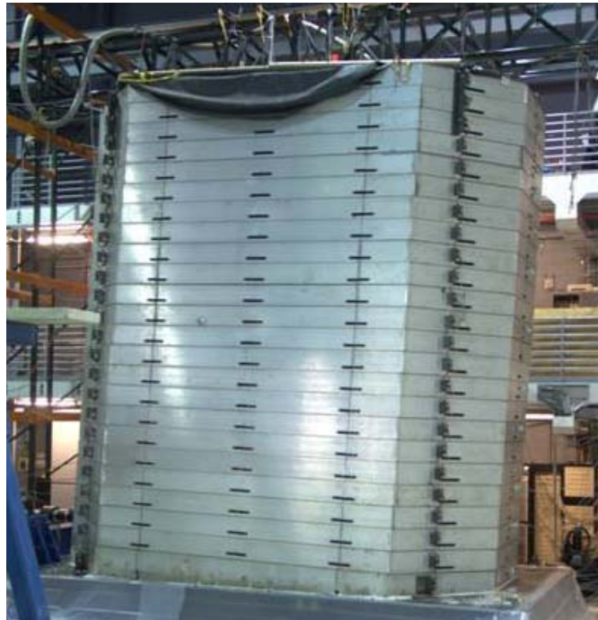
Figure 16. 2-degree inclined laminar box before Test SG-1.
