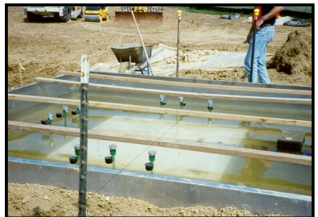
Figure 19. Sealed double-ring infiltrometer test in progress.
